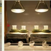
Figure 4: Several "drying" steps in between adding acids are necessary after collecting for specific isotopes.
